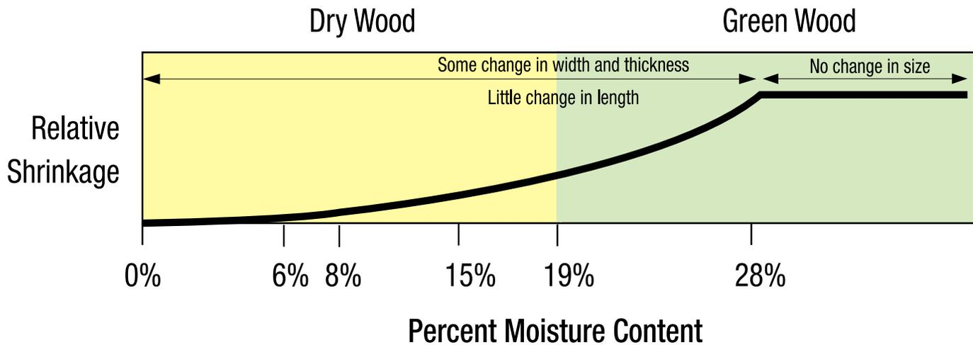
*Dry lumber has already done most of its shrinking, making construction easier. Lumber can either be dried naturally in the air (and then stamped "S-DRY" for surfaced-dry), or it can be dried with heat, in a kiln (stamped "KD" or "S-DRY").*
